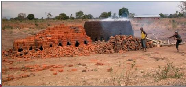
Brick-making using woody materials
